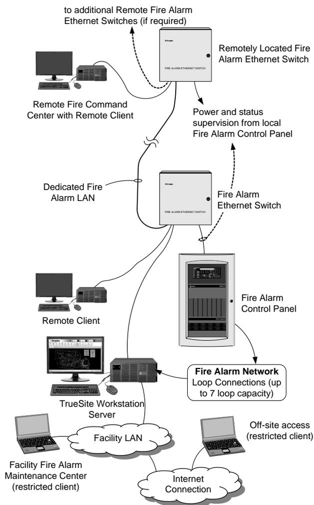
Fire Alarm Ethernet Switch Connection Reference
