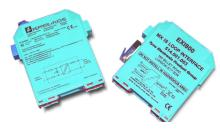
The EXI800 can detect a short circuit on the left-loop, the right-loop, or the IS loop and will isolate the offending loop connections from the other loop connections. The IS loop output of the EXI800 interfaces with the Pepperl+Fuchs KFD0-CS-Ex1.54 Galvanic Isolator, supplying loop voltage and signalling currents to the Intrinsically Safe loop.
